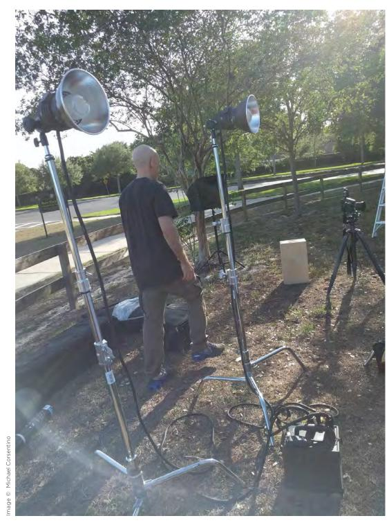
A 1,200-watt second battery-operated pack with the power split between two heads provided all the power I needed to evenly illuminate the scene.
